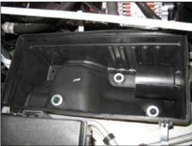
g. Remove the three bolts securing the bottom half of the air box to the vehicle.
