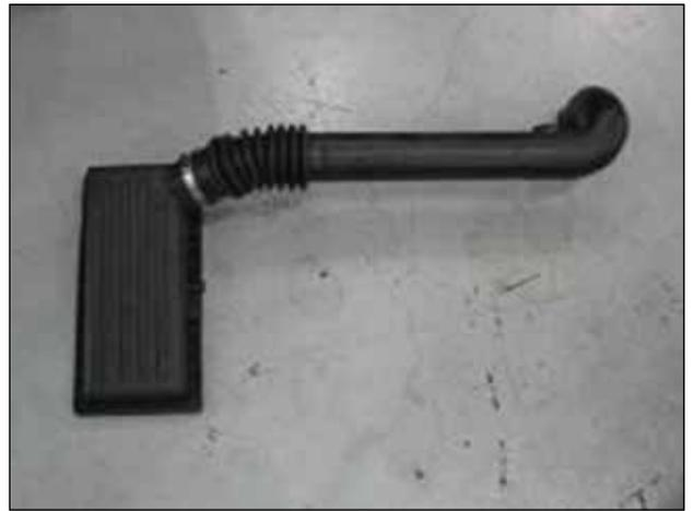
f. This is the intake tube and air filter lid after removal from the vehicle.
