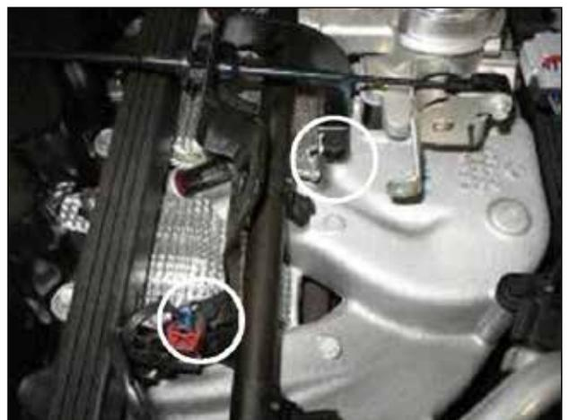
j. 2000-2006 Vehicles: Remove the 2 bolts on the throttle body linkage and replace with the supplied bolts and spacers.
