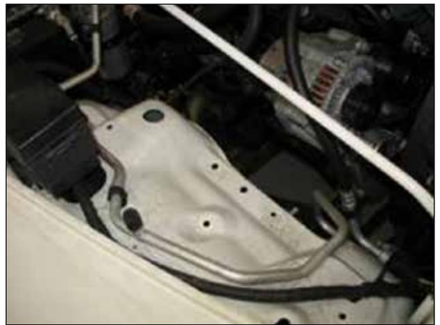
h. The factory air box housing removed.
