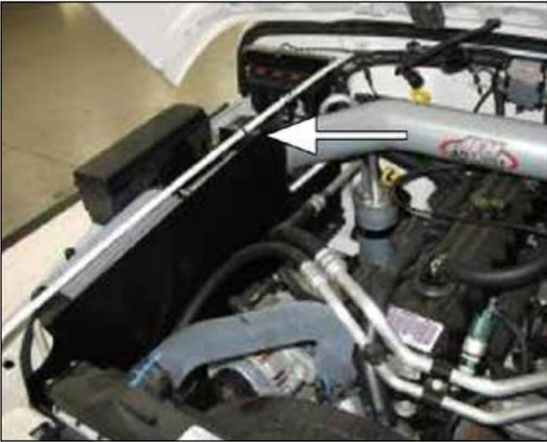
I. Attach the AEM® Dryflow™ air filter to the end of the intake pipe using the #52 hose clamp. Use the supplied zip tie to secure the heat shield to the support bar.
