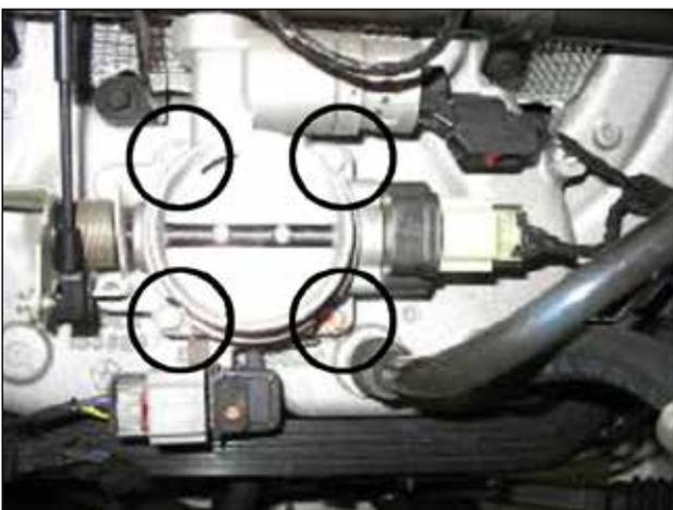
i. Remove the four bolts securing the throttle body to the intake manifold. After removal of the four bolts, place the throttle body spacer between the throttle body and the intake manifold. Install with the supplied gaskets and bolts, refer to the diagram on page 2 for the gasket placement.
