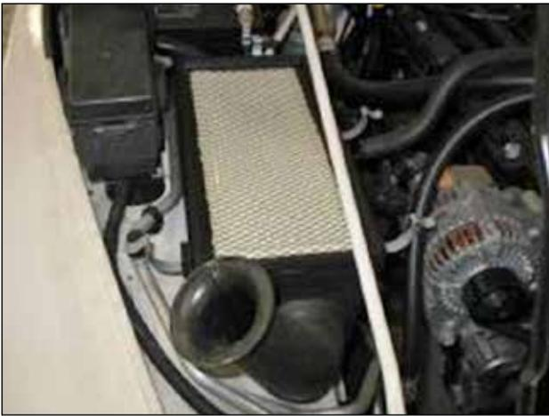
e. Remove the air filter lid from the air filter housing. Unclasp the four retaining clasps. Also be sure to disconnect the crank case breather hose from the lid.
